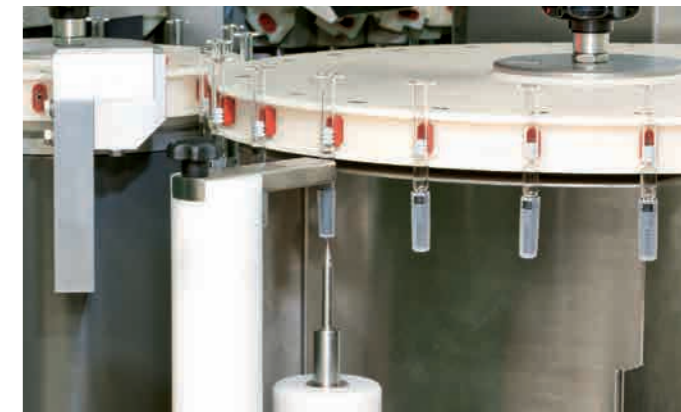
High voltage reliably identifies defects in the needle shield by way of a spark caused by the conductivity of the protruding needle. Tests show that this method can even detect weak points in syringes in which the needle is surrounded by a rigid plastic shield (RNS).
